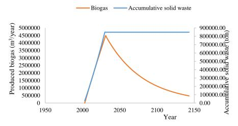
Figure 2. The aggregated gas rate and produced biogas in the Marvdasht landfill
