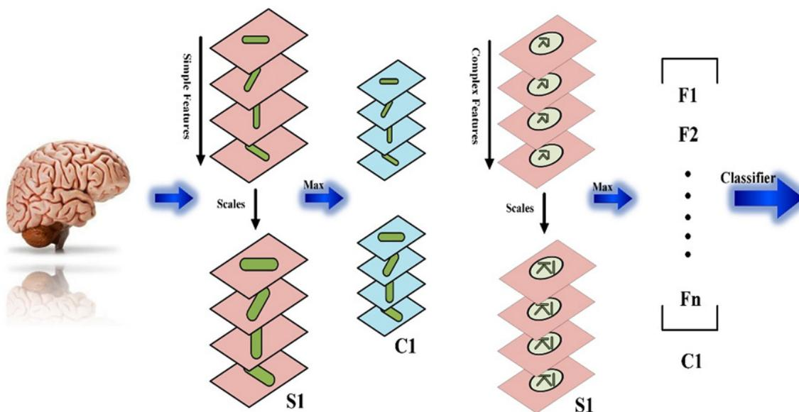
Figure 3. The Architecture of the network used in Mutch's method.
