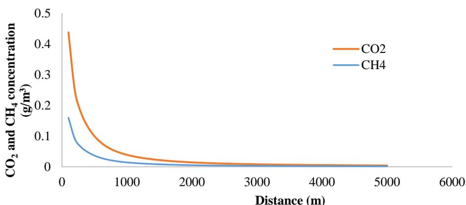
**Figure 7:** Concentration shifts of carbon dioxide and methane with changes in distance from the landfill
