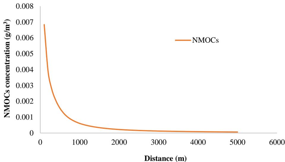
**Figure 8.** The concentration shifts of NMOCs with changes in distance from the landfill
